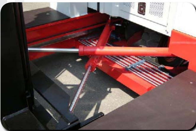
BP utilizes a cross system of hydraulic pistons rather than chains to extend and retract the mast for smooth even positive control.
