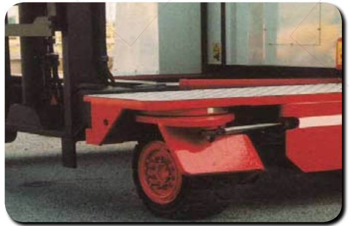
3-driven and steered wheels provide optimum performance and control in tight quarters. The vehicle steers in forward-reverse & side-side mode.
