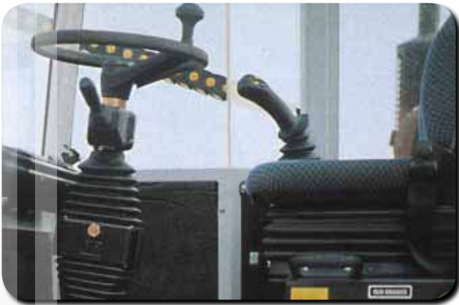
Multifunctional finger tip joystick control of the hydraulics. Rigid mast made from manganese extruded steel.
