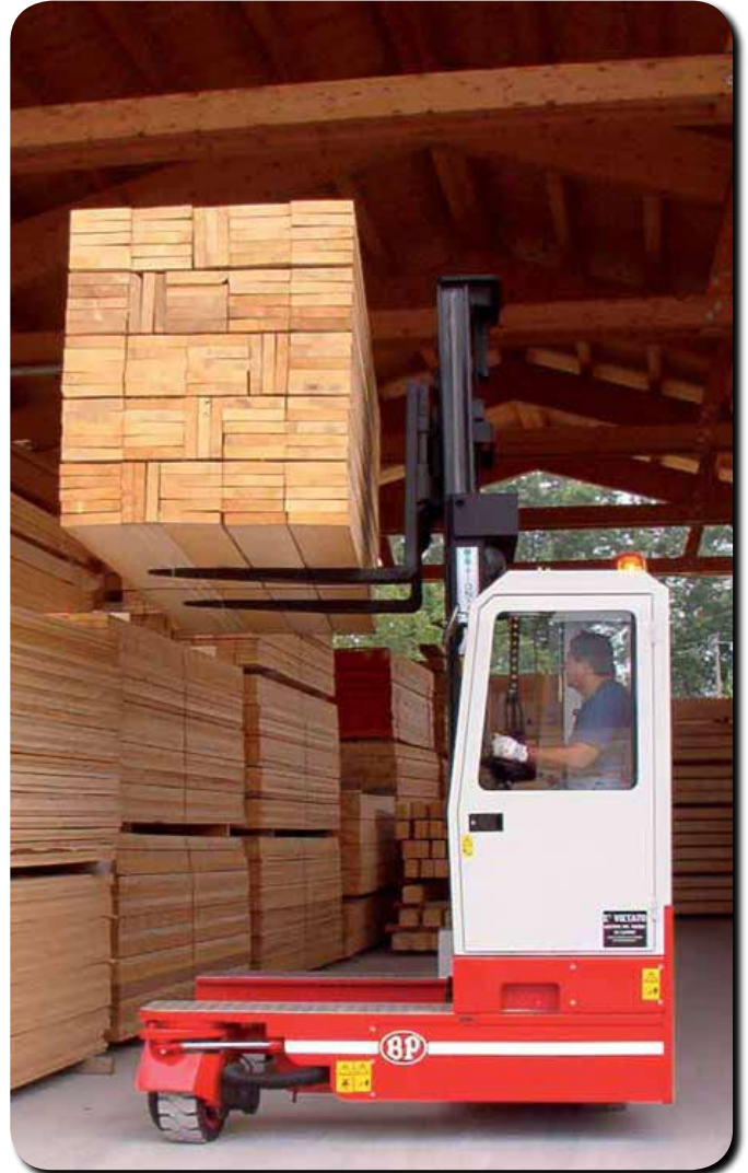
3-driven and steered wheels provide optimum performance and control in tight quarters. The vehicle steers in forward-reverse & side-side mode.
